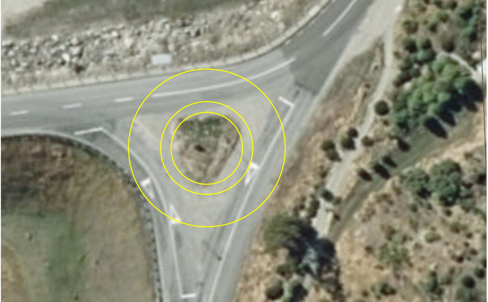
Figure 4: Central Island and Outer Diameter of State Highway 84 / Anderson Heights Roundabout Overlaid at Domain Road / Capell Avenue Intersection
