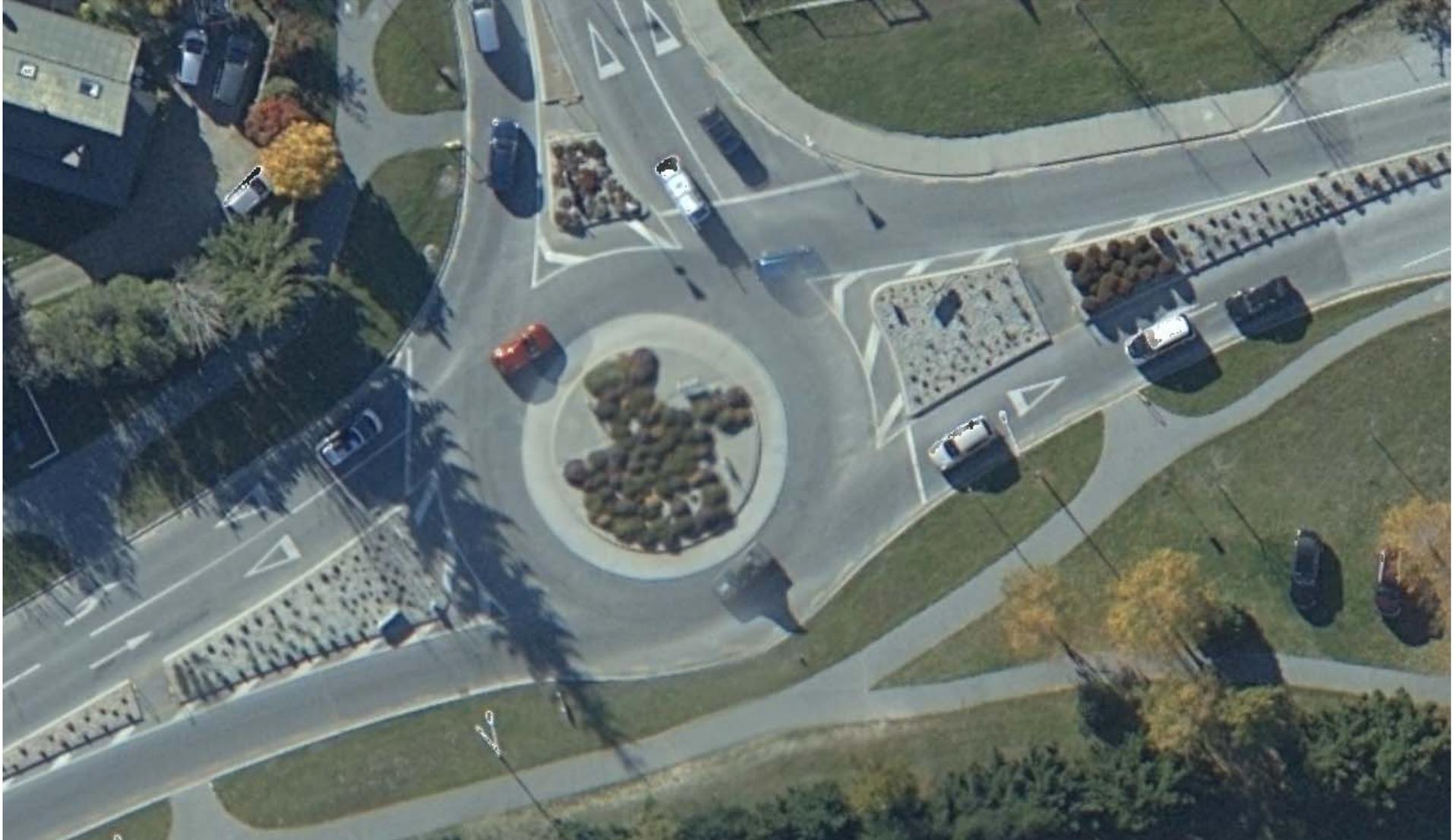
Figure 2: 30m Diameter Roundabout at State Highway 84 / Anderson Heights
