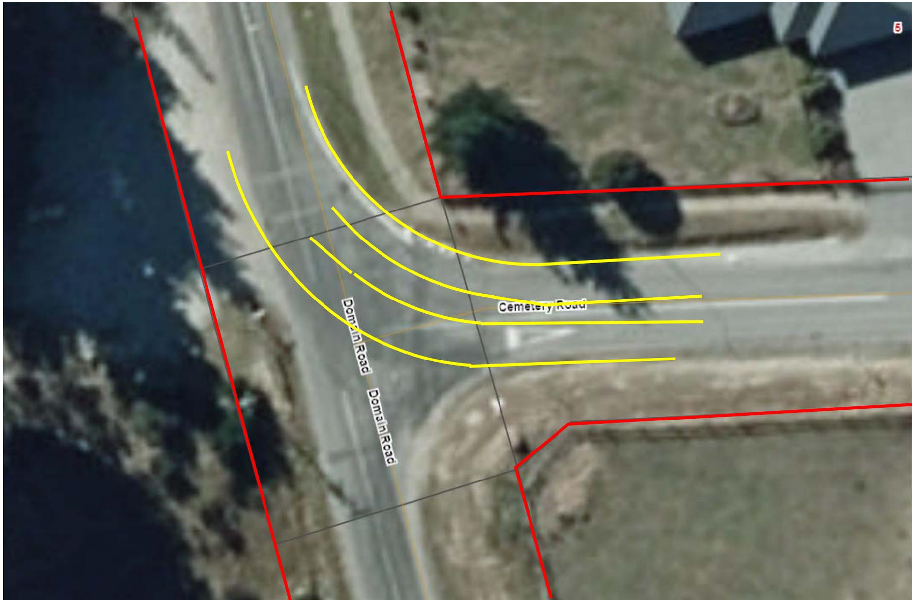
Figure 5: Curve Markings at Frankton Road / Stanley Street Intersection Extended to Align with Domain Road
