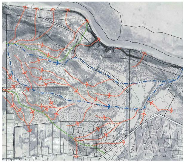
Figure 4 - Stormwater runoff paths (see Appendix 3)
