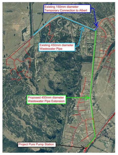
Figure 3 Existing and Proposed Wastewater Reticulation in Aubrey Road
