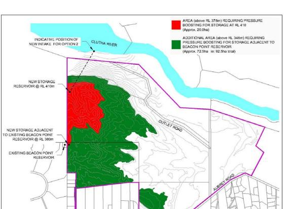
Figure 2 Map showing areas requiring boosting of water supply and indicative layout for Option 2.
