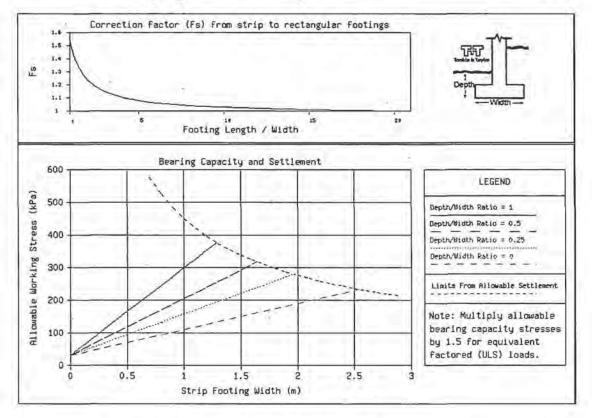
From Figure 7.2 it can be seen a working bearing stress of approximately 120kPa is recommended for a 400mm wide by 400mm deep strip footing bearing on River Gravels or Engineered Fill overlying River Gravels/Schist Bedrock. This corresponds to a factored (ULS) bearing capacity of approximately 180kPa and a geotechnical ultimate bearing capacity of 360kPa.
