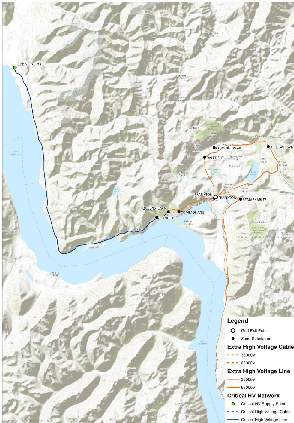
Frankton Sub Transmission Network and Critical Distribution Electricity Lines
