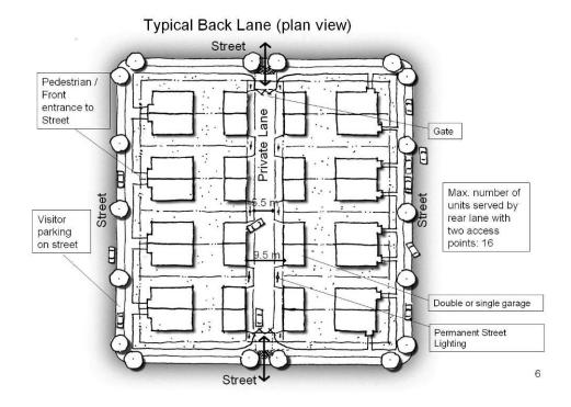
The above diagram is an example of how a back lane can be used to provide access to garages at the rear of the property. Note: this diagram is indicative of concepts only. There is no guarantee the design shown would prove appropriate to the applicant or satisfy all requirements to gain consent.
