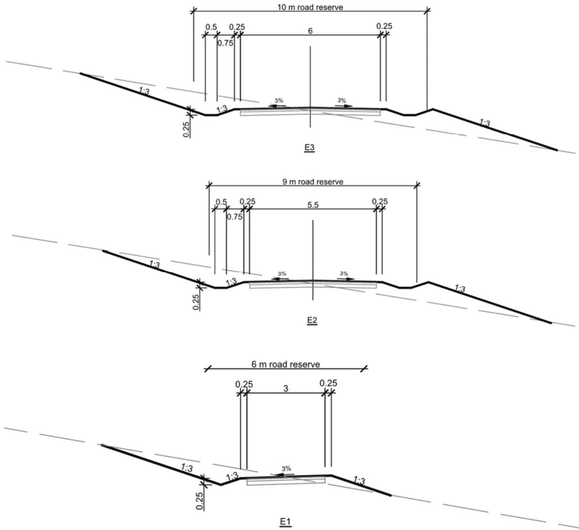
Figure 4 Typical sections for type E1, E2 and E3 roads complying with QLDC LDSC
