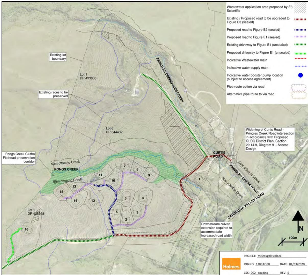
Figure 3 Proposed roading upgrades in accordance with QLDC LDSC
