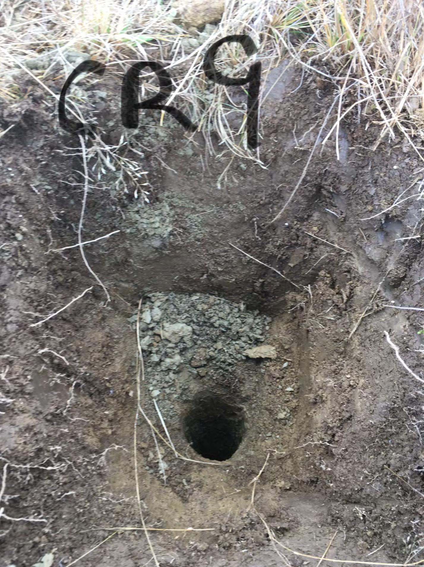
Test Pit for CR9. Depth of hole dug to 0.4 mbgl and extended to 1.5 mbgl with auger.
