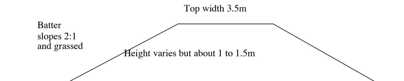
**Figure 3.6: General minimum dimensions for stopbank top width and batter slopes**
