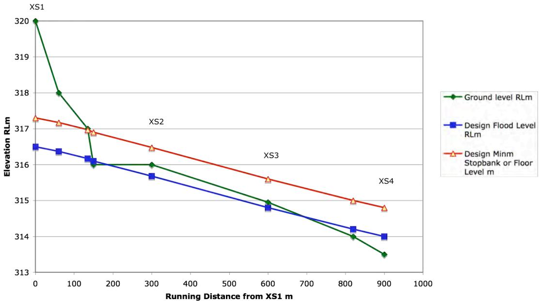
**Figure 3.5: Recommended stopbank OR hardfill levels compared with existing ground level on left bank**
