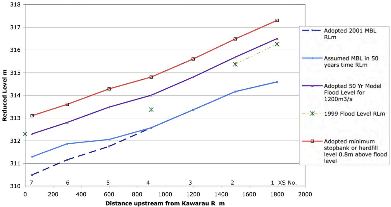
**Figure 3.4: Recommended stopbank OR hardfill levels to be 0.8m above 1% AEP floods by 50 years time after smoothing of 1200m<sup>3</sup>/s grade line**
