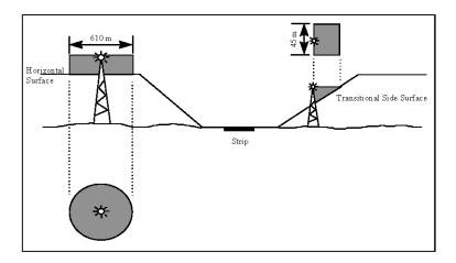
Figure C.2 - Shielding Transitional and Horizontal Surfaces
