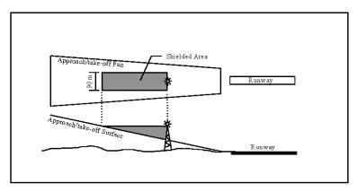
Figure C.1 - Shielding Approach and Take-off Surfaces
