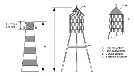
H is less than 45 m for the examples shown above. For greater heights intermediate lights must be added as shown below.
