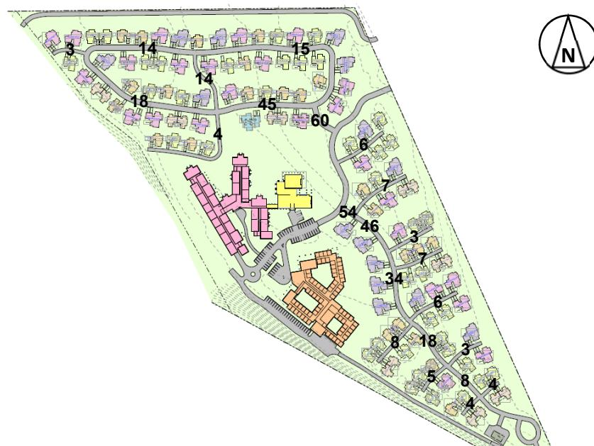
**Figure 6: Expected Loading (Residential Units) on Internal Roads**
