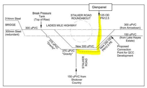
Figure 3.2: Schematic Diagram of Sewer Pipework at the Western End of Ladies Mile
