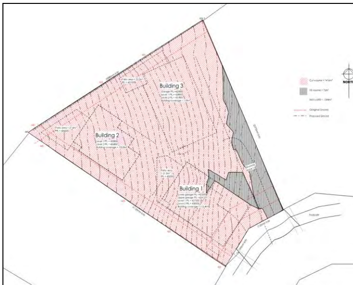
Proposed earthwork cut & fill
