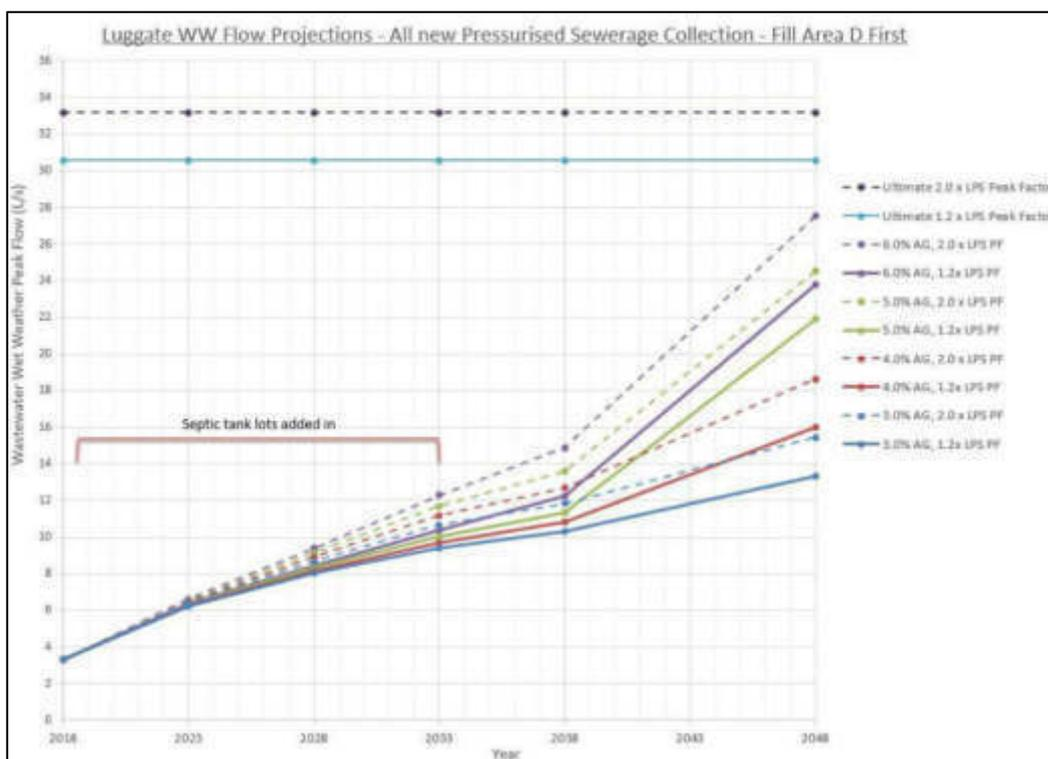
**Figure ES3: Peak Wet Weather Wastewater Flow Projections Pressurised Sewer Option – Area D Developed First**
