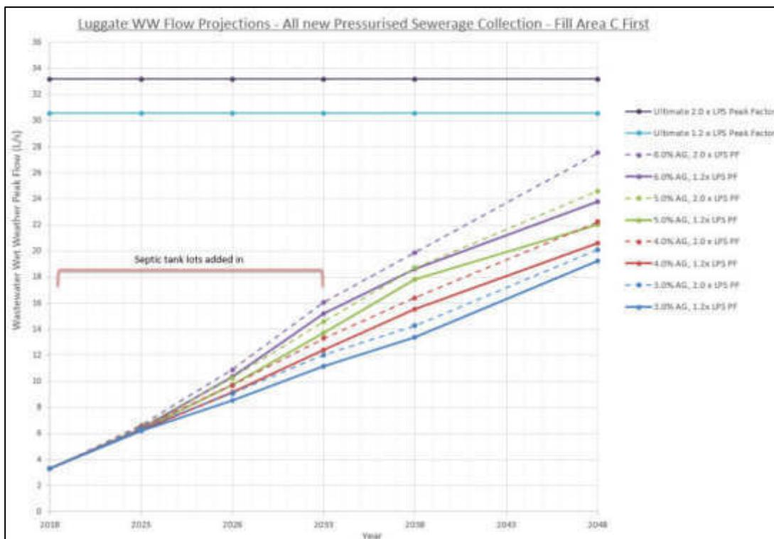
Figure ES2: Peak Wet Weather Wastewater Flow Projections Pressurised Sewer Option – Area C Developed First
