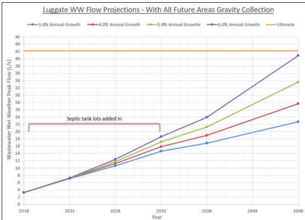
**Figure 6.1: Peak Wet Weather Wastewater Flow Projections for Conventional Gravity Sewerage System for Luggate**
