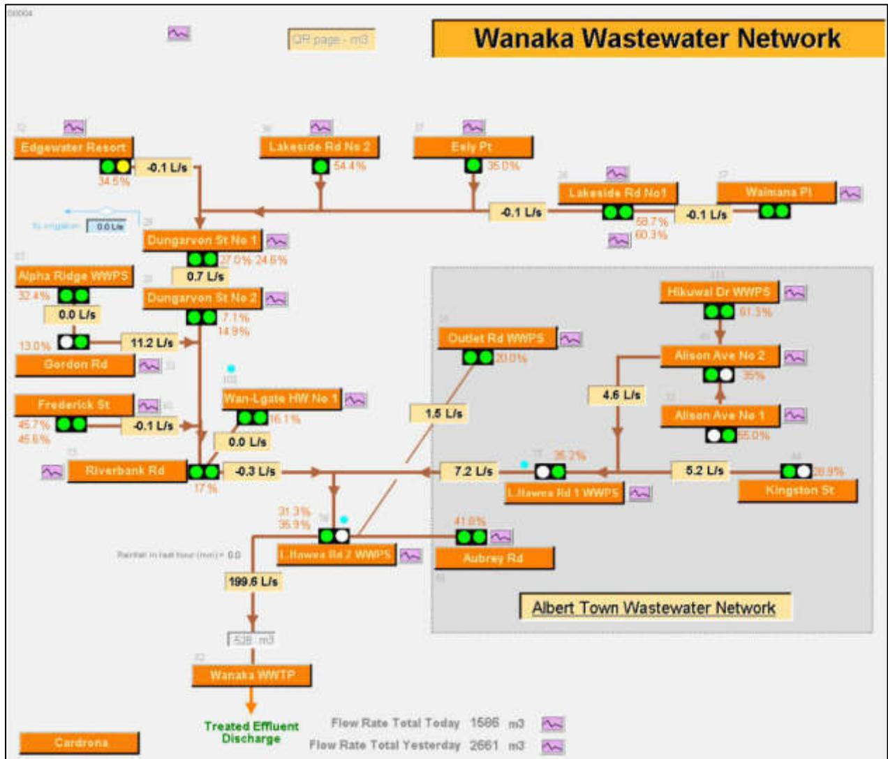
Figure 3.2: Schematic of Wanaka Wastewater Network Pumping Stations
