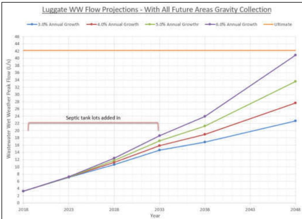
Figure ES1: Peak Wet Weather Wastewater Flow Projections for Luggate – Conventional Gravity Reticulation Option
