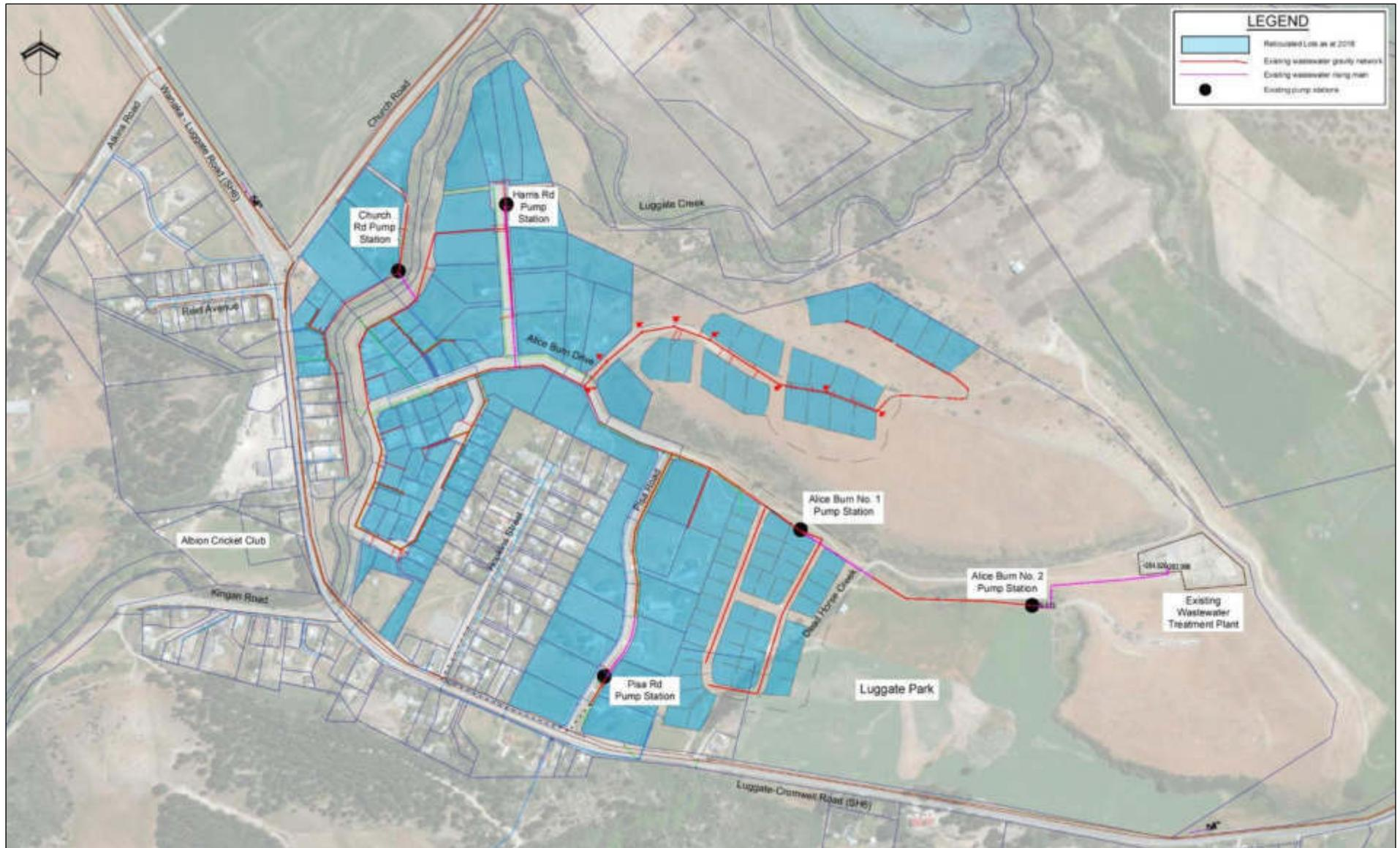
Figure 3.1: Plan of Existing Sewerage System at Luggate
