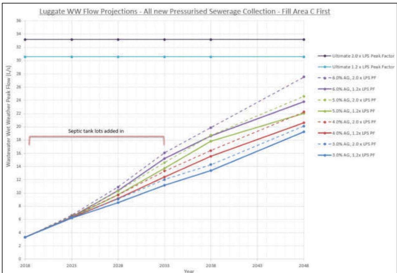
**Figure 6.2: Peak Wet Weather Wastewater Flow Projections for Pressurised Sewerage System for Luggate – Fill Area C (Luggate Park) First**
