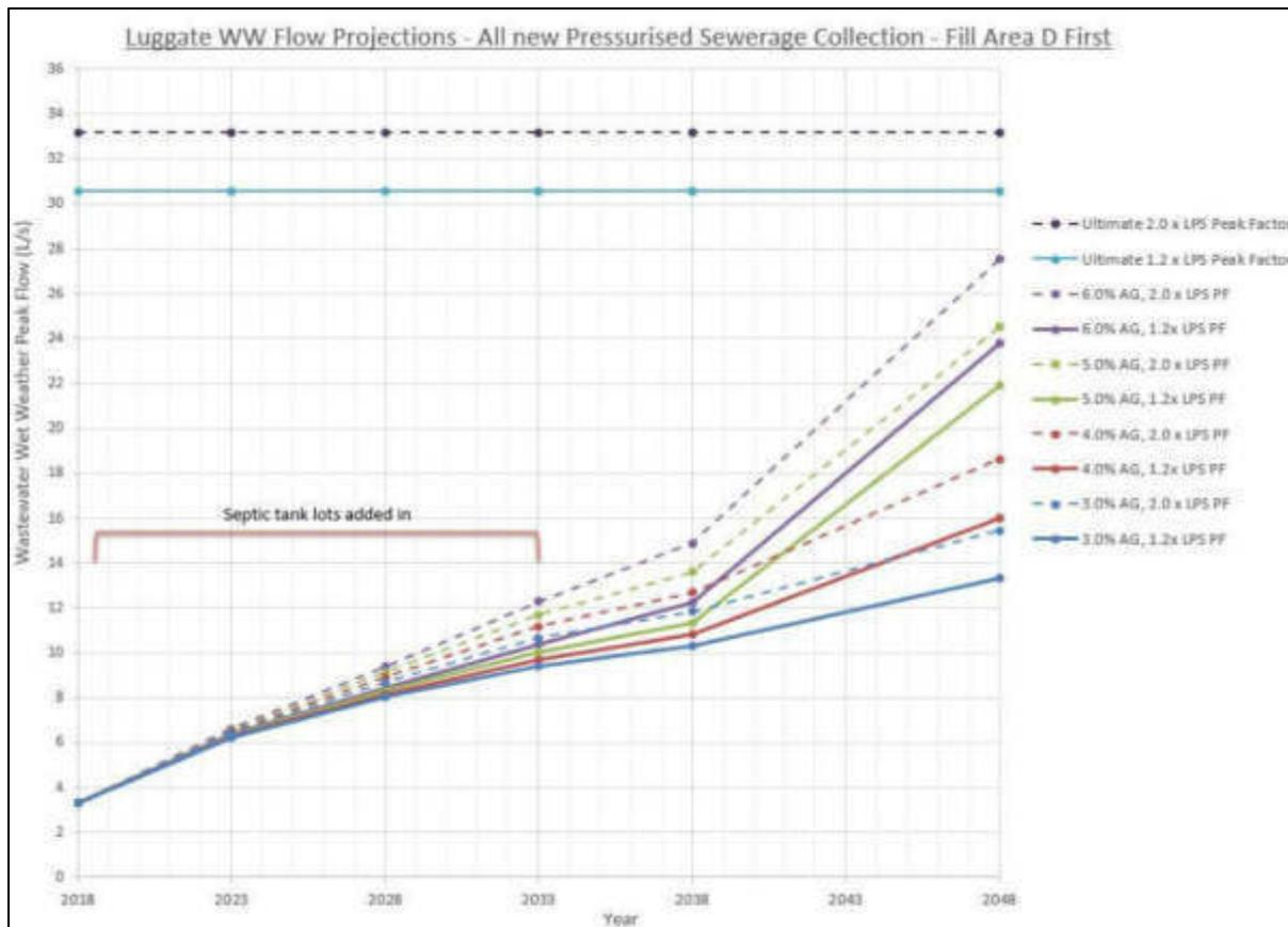
**Figure 6.3: Peak Wet Weather Wastewater Flow Projections for Pressurised Sewerage System for Luggate – Fill Area D First**
