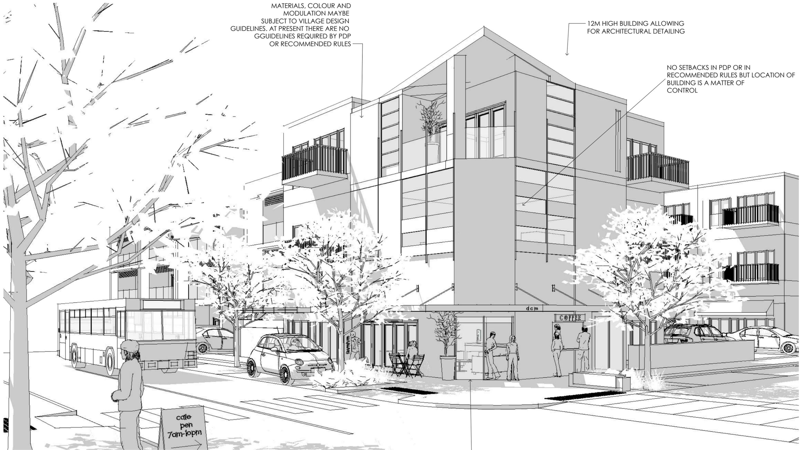
This sketch shows a 3 storey, 12m high mixed use (commercial/retail/residential) building built up to the street frontage with car parking placed behind. The building has a minimum 3.5m ground to floor (next) height to allow future flexibility of building use. The building has active frontages on both sides providing an improved experience for pedestrians (compared to blank walls and carparking) and allowing businesses to 'spill out' onto the footpath
