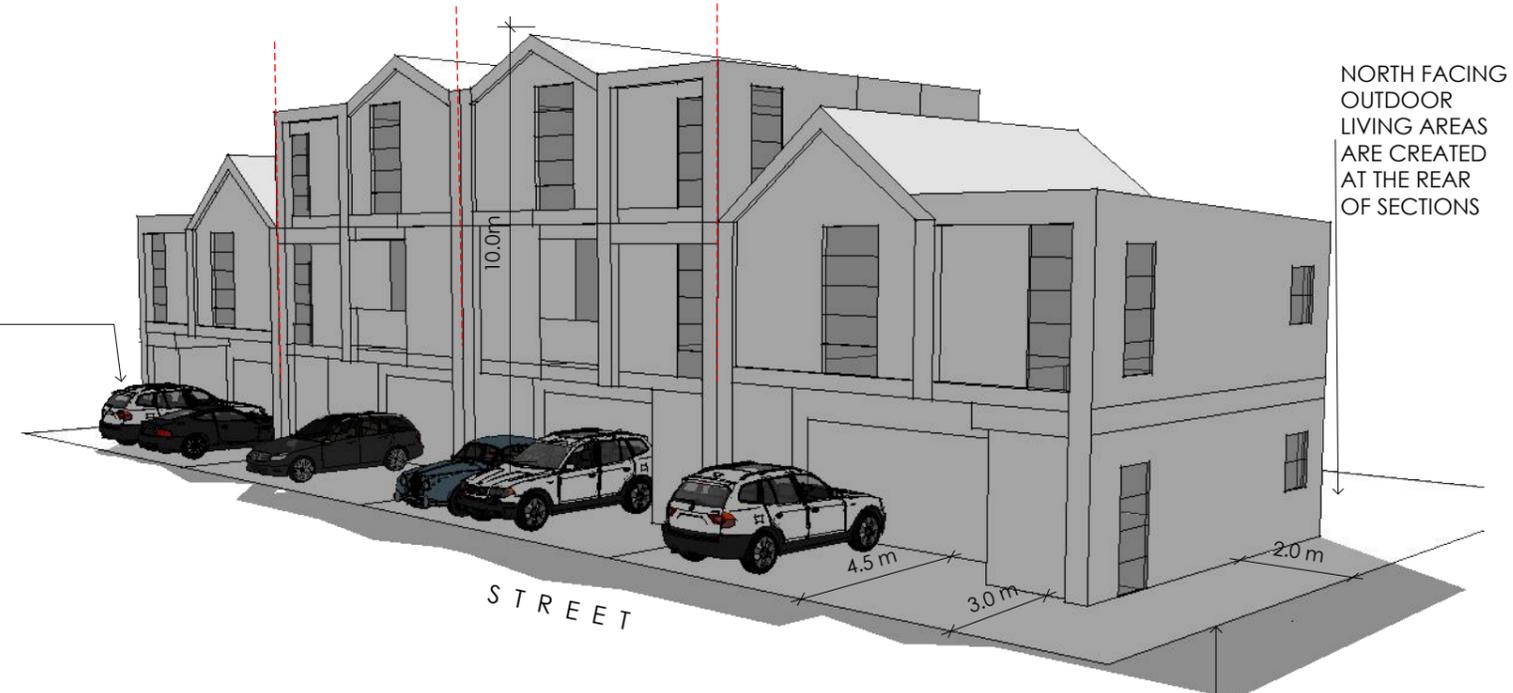
THE PLACEMENT OF GARAGING/PARKING IN THE FRONT YARD CAN RESULT IN A POORLY DESIGNED STREETScape DOMINATED VISUALLY (AND PHYSICALLY) BY CARS.
