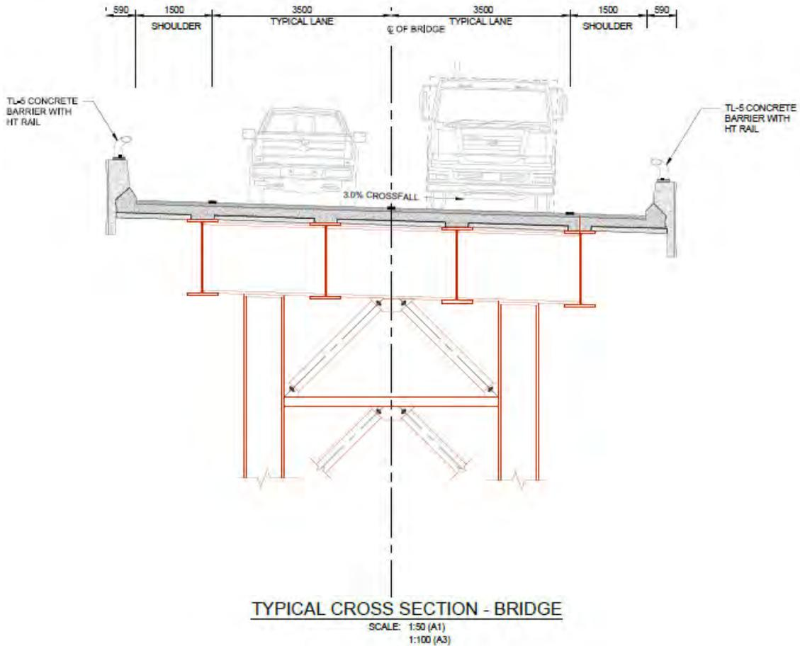
Figure 25 Recommended Option Road Bridge Cross Section
