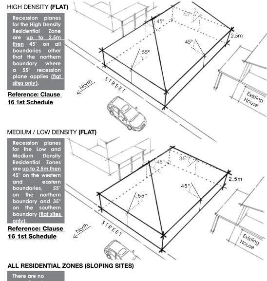
recession planes on sloping sites (except for accessory buildings). Sites are defined as sloping where the ground slope exceeds 6° across the extremities of any building elevation. (submitter 3016)
