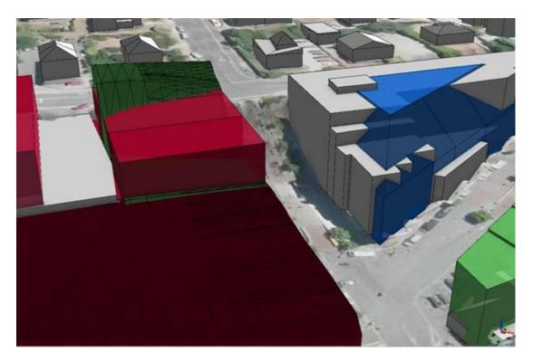
Key: Green 12m rolling height plane; Pink 7 m above 327.1; White Sofitel existing built form; Blue 10 m recession plane. New modelling showing the submitters' proposed 7m horizontal plane.
