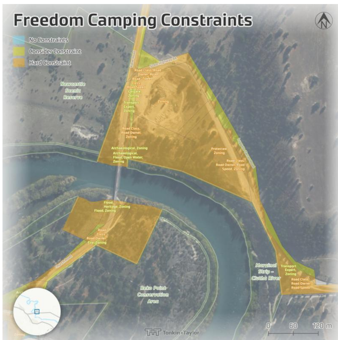
Figure ii: Example of mapped attributes present on the land, with related constraints. Each parcel of land is subdivided into smaller areas based on where particular constraints are mapped as present.
