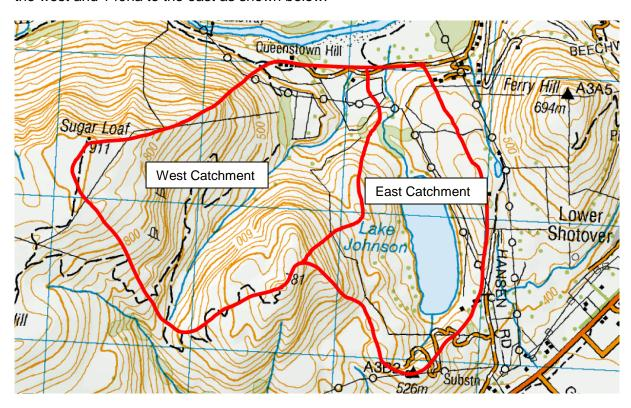
The run-off from the development area within the eastern catchment does not discharge to Lake Johnson. Instead the development is located within the catchment at an elevation and location that all stormwater will be discharged to the outlet creek of Lake Johnson.
