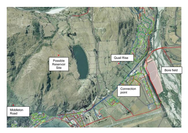
Sizing of the reservoir should also be carefully considered as this could help eliminate peaks in the demand. This would then allow for a lower peak flow of water to be taken from the existing QLDC system.
